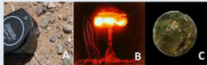
Fig 1: Nuclear fallout originates from soil swept into the fireball during the nuclear explosion. Figure A is an image of soil found near Trinity ground zero. This soil is swept up by the fireball, represented by image B, where it is subject to thermodynamic conditions that result in the formation of aerodynamic fallout, image C.
