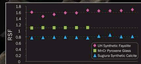
Figure 4: Relative sensitivity factors for measured minerals. The average values are denoted by the dashed lines: approx. 1.6 for synthetic fayalite, 1.1 for a Mn,Cr pyroxene glass, and 0.8 for synthetic calcite.
