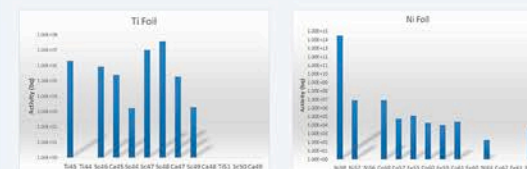
The modeled isotopes produced in Ti and Ni foil in units of activity. ENDF cross-sections were used to calculate the production
